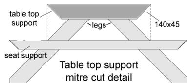
So, using the two 2400mm lengths of 140mm x 45mm, cut four table top supports to 1015mm (or to the measurement you made), and mitre the ends, as you did for the seat supports.
