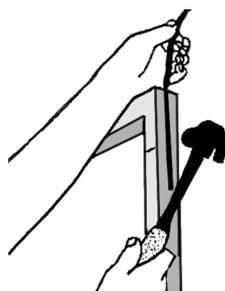
Adjust the cord if necessary, then insert two or three more fixing nails below the first one.
