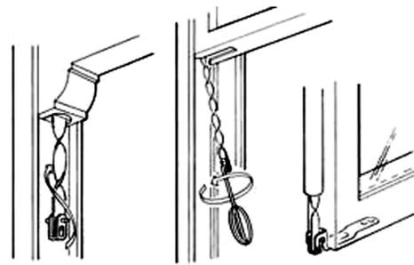
Pull the mechanism down about 150mm without allowing it to untwist and lose the spring's tension. Turn the tool two or three times anti-clockwise to add tension, then hook it back in place.
