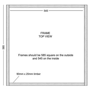
Continue making up sets of frames, stacking each squarely on top of the other as you go. You should end up with a stack of five frames that is around 450mm high.
