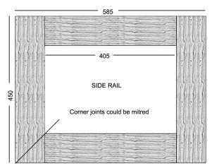
It would be a good idea to measure the stack of frames before cutting the rails. You could use a mitre joint on the rails if preferred.
